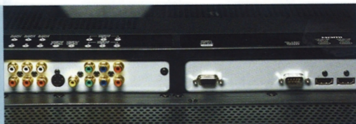
Two component video inputs and two HDMI sockets mean the Fujitsu is well connected. There are no Scarts, though
